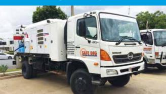
Jetting uses high pressure water technology passing through a hose & nozzle to effectively clear conduits of debris, scales, encrustation or dislodge sand/sediment & move it to a point where it can be expunged from the pipeline system.
